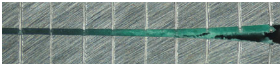
Fig. 3 Damage process of an adhesive. Crack tip to the right; to the left undamaged adhesive with a nominal thickness 0.2 mm. Specimen marked with vertical scratch marks every millimeter
